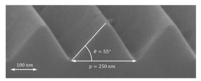
Figure 1. SEM characterization of nanopatterned V-groove silicon substrate.
